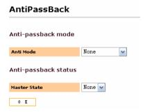
2. The selections of anti-pass back mode. There are 4 selections: out antipassback, in antipassback, in&out antipassback, no antipassback, none and save.
