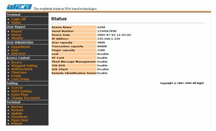
The device information includes: device name, serial number, device date, IP address, user capacity, record capacity, finger capacity; as well as the status information of some functions.
